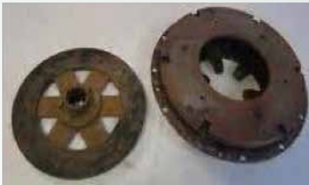
Original Clutch plate and Pressure plate. NOTE: The original Clutch plates don't have springs.
