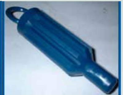
Clutch plate/disc alignment tool
