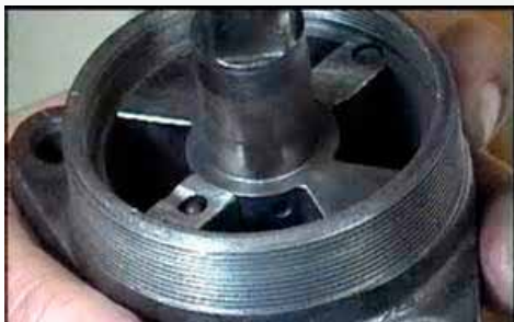
Base Stationary wings and Moveable Wing Shaft (Note check ball holes in the Stationary Wings, the hole in the Moveable Wing Shaft and the threaded area for the Inner and Outer Covers)
